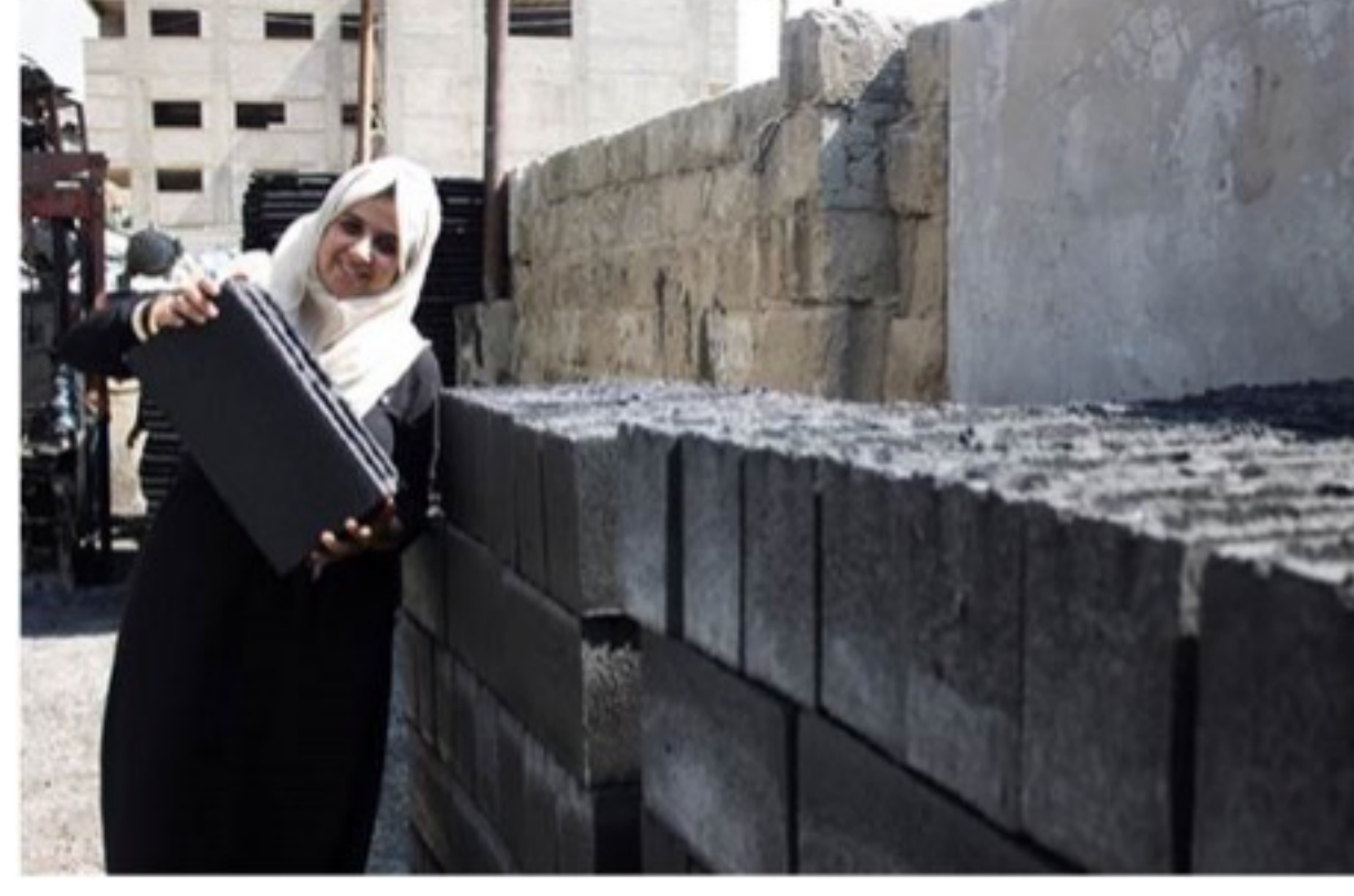
Majd Mashharawi (GRC Staff, 2018) is a founder and CEO of Gaza startup, Green Cake, that designs bricks made of ash and rubble from local buildings destroyed by war. An inexpensive alternative to cement, the technology is helping to rebuild Gaza and create opportunities for female entrepreneurs.
